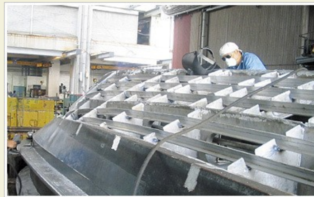
Replacement of Hull Plate 政府船塢船體維修
